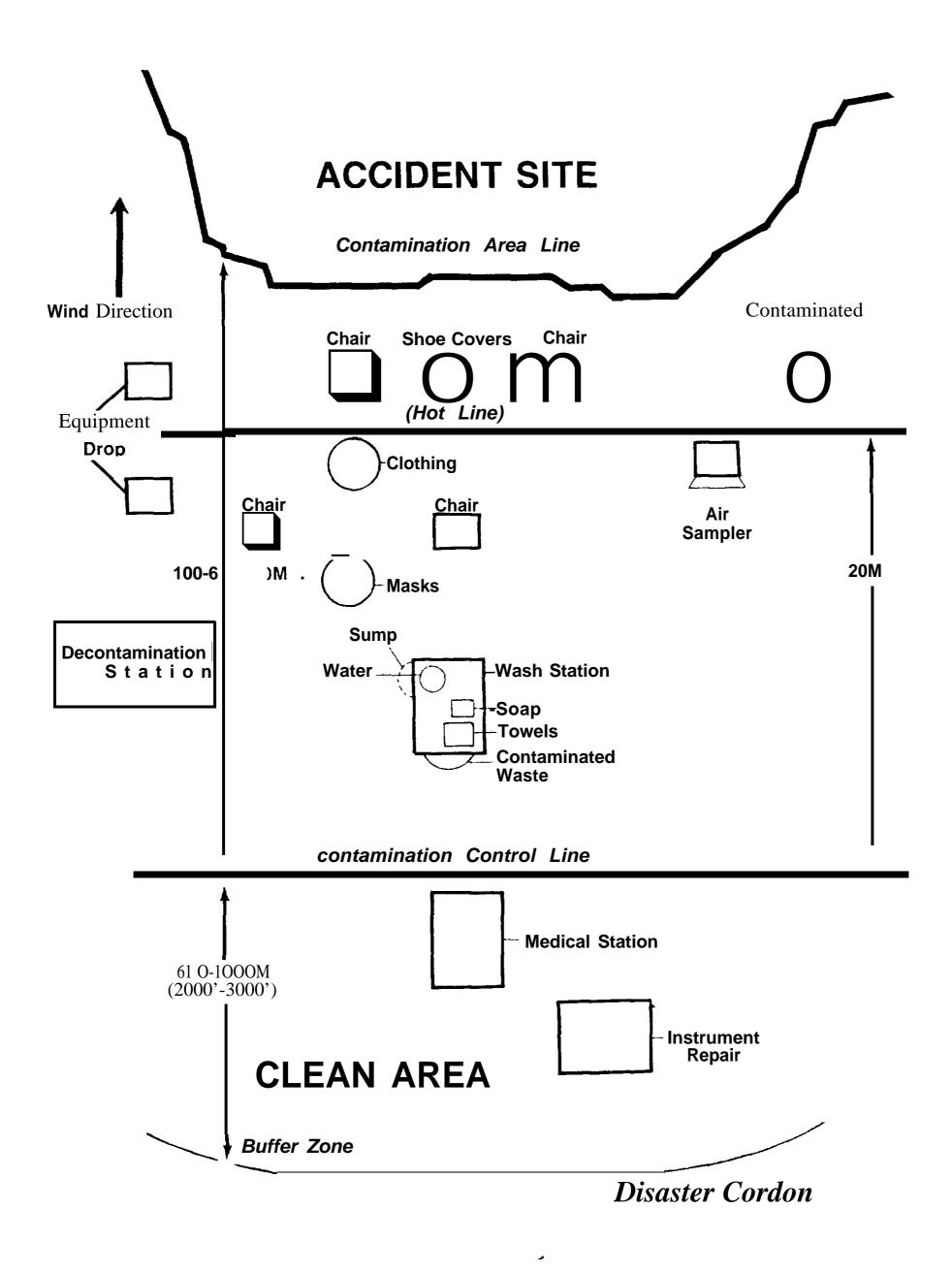
Figure 7-1. Contamination Control Station (Example).
