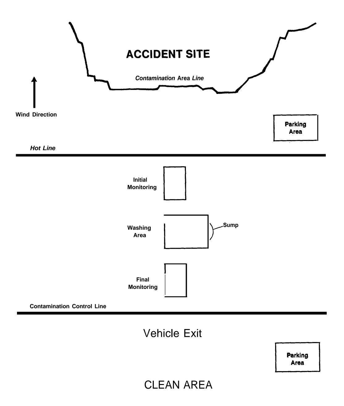
Figure 7-2. Vehicle Contamination Control Station Example.
