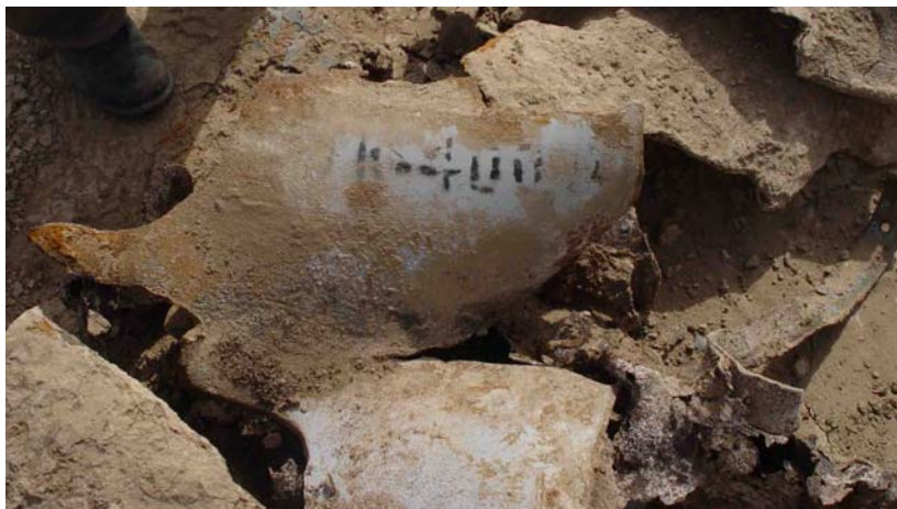
Figure V.XI.V Recovered R-400 Bomb Fragments in 2003 with markings such as the bomb type (left) and the black stripe (right).
