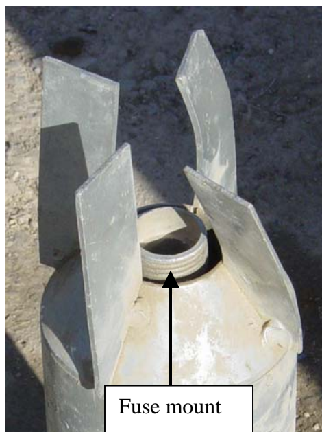
Figure III.X.XXIIIA Base of the sub-munition showing fins in place and rear of the
