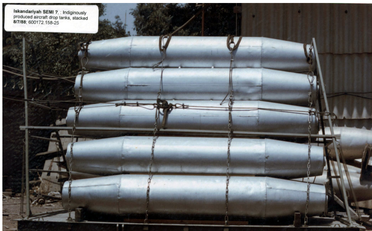
Figure III.X.XXIV indigenously produced aircraft drop tanks
