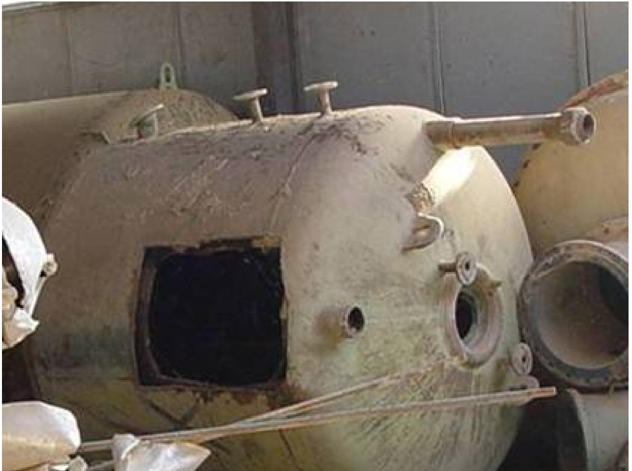
Figure III.XI.XXVI A tank destroyed by cutting out a hole
