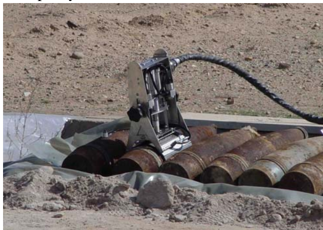
Figure III.X.IIIA Remote drilling into a mustard filled projectile with MONICA
