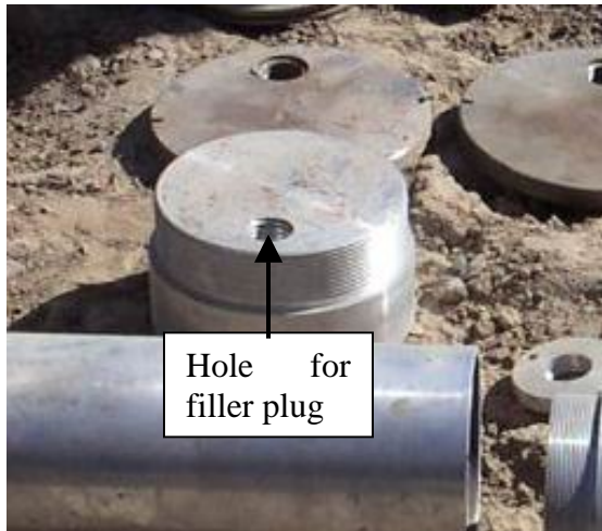
Figure III.X.XXXIIA Base plate for 107mm warhead
