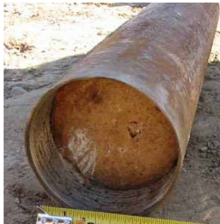
Figure III.X.XVA Base of warhead showing TNT filler
