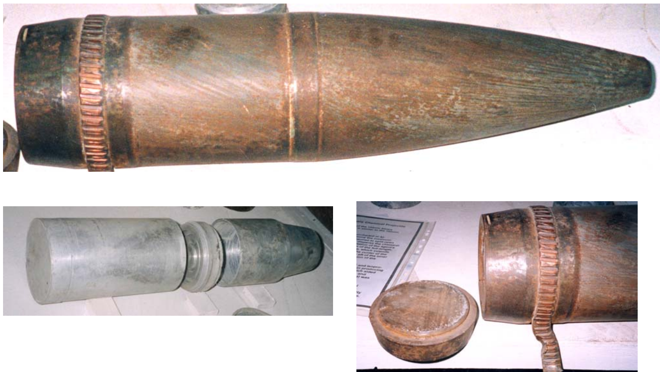
155mm Extended Range Full Bore Boat Tail (ERFB-BT) Binary Sarin
