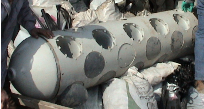
Figure III.X.LIIIA Nasr 28 cluster bomb showing covered and uncovered ejection
