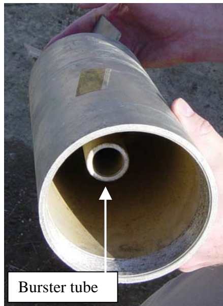
Figure III.X.XXIA Burster tube inside sub-munition
