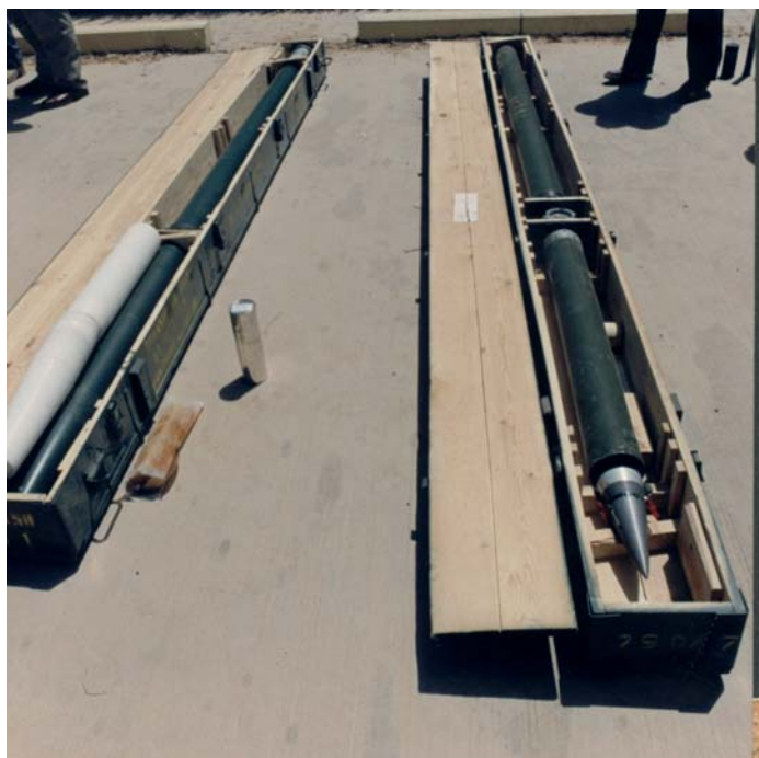
Figure III.X.IX “SAKR-30” type 122mm rockets; warhead, motor and one section of the agent container
