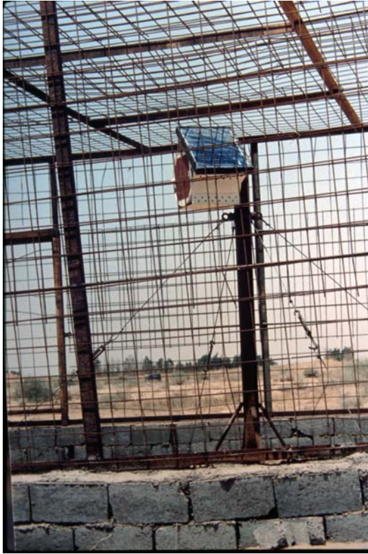
Figure III.XI.XXXI Air samplers installed at Muthanna site (automatic, driven by a solar panel)
