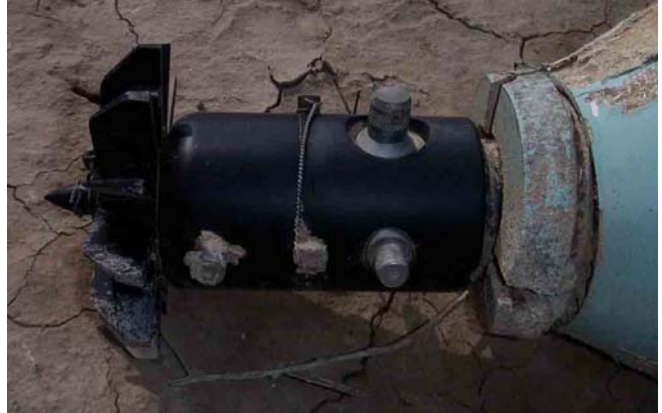
Figure III.X.XLIVA Airburst fuse on a CB 250 cluster bomb
