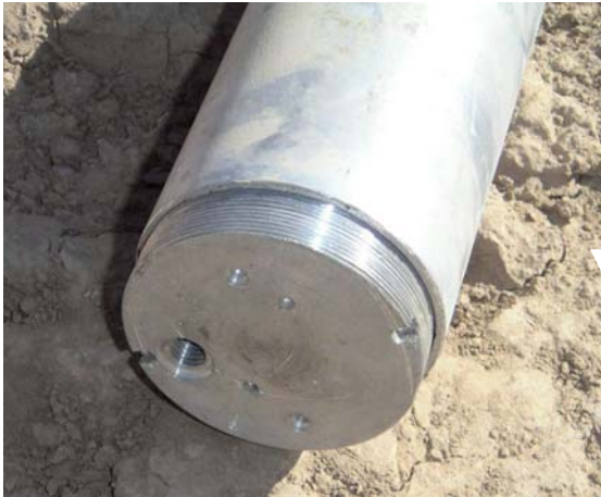
Figure III.X.LXIIA Base assembly of 81 mm warhead. Note- base plug is not fully in place
