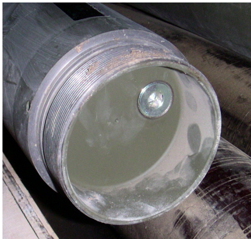
Figure III.X.IXA Base of “Firos” type warhead
