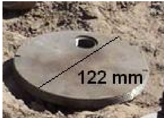
Figure III.X.XIXA Rear side of base plate showing possible filler
