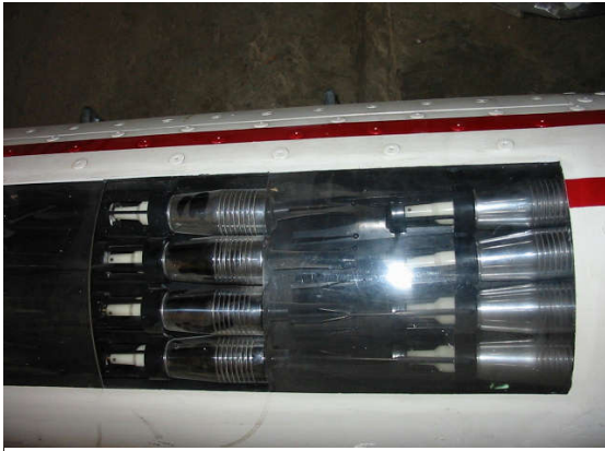
Figure III.X.XLIIIA Conventional sub-munitions in the CB 250 cluster
