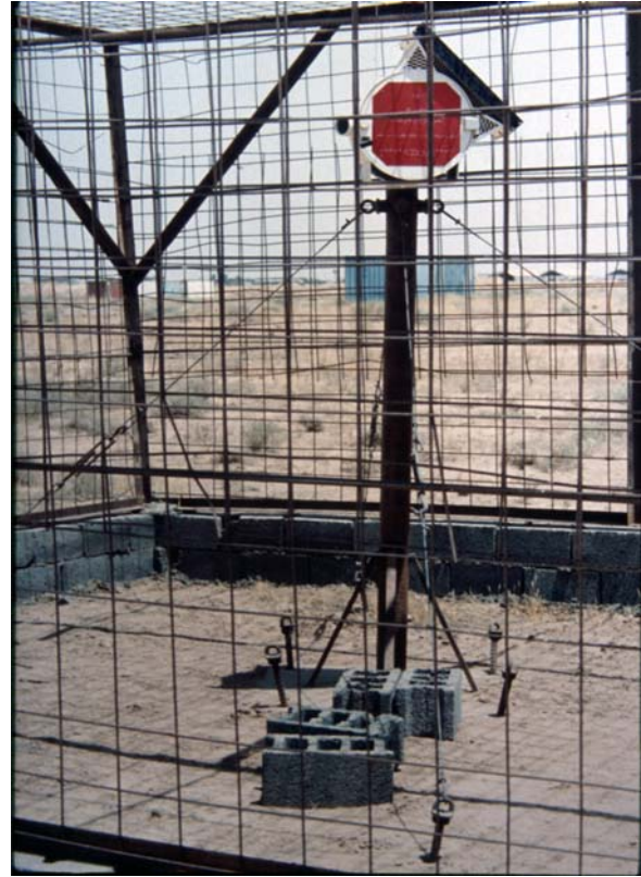
Figure III.XI.XXXI Air samplers installed at Muthanna site (automatic, driven by a solar panel)
