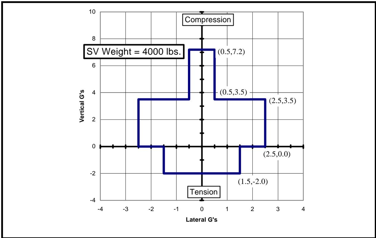
Figure 19 - MLV-S Quasi-Static Load Factors
