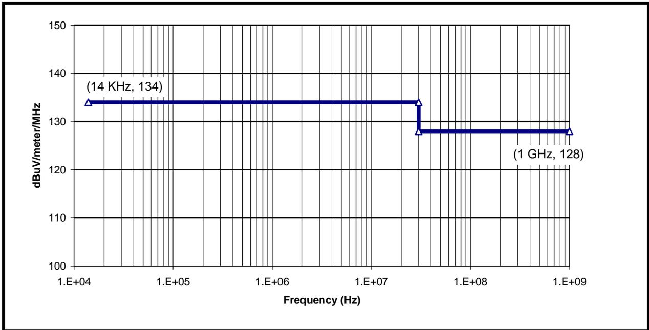
**Figure 12 - Maximum Allowable Broadband SV Radiated E-Fields**
