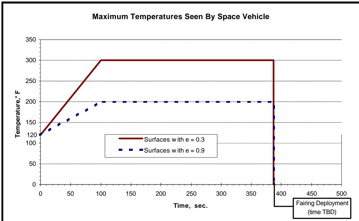
Figure 18 - Maximum PLF Inner Surface Temperatures
