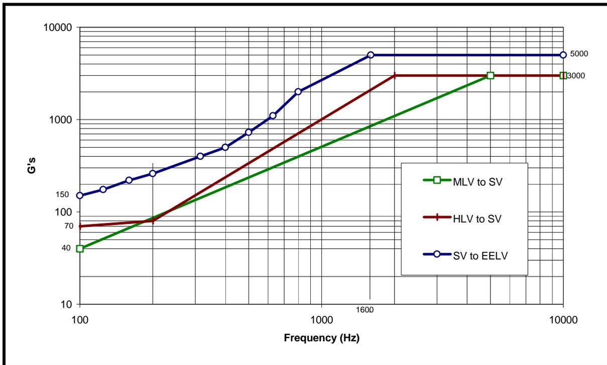
**Figure 24 - EELV Maximum Shock Levels**
