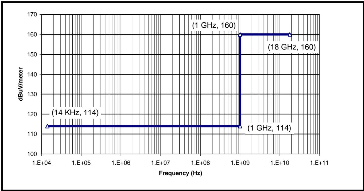
**Figure 11 - Maximum Allowable Narrowband SV Radiated E-Fields**
