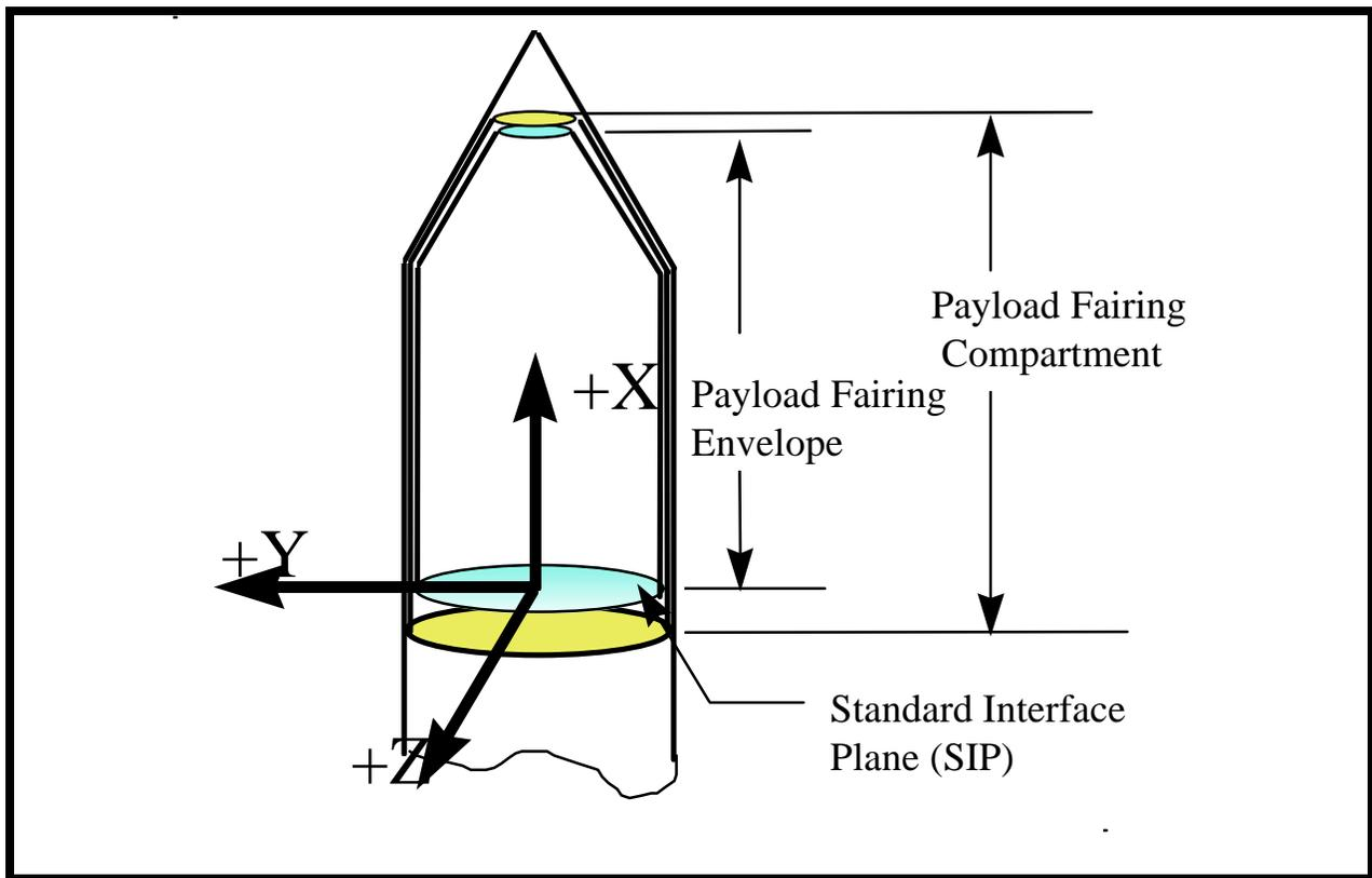
**Figure 1 - EELV Standard Interface Coordinate System**
