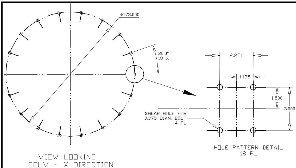
**Figure 4 - Large diameter (173'') payload interface**
