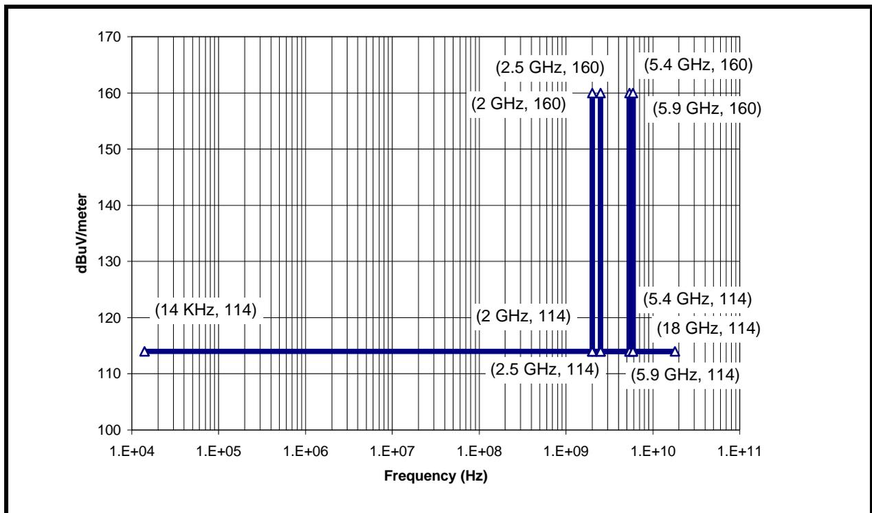
Figure 13 - Maximum Allowable Narrowband LV Radiated E-Fields.
