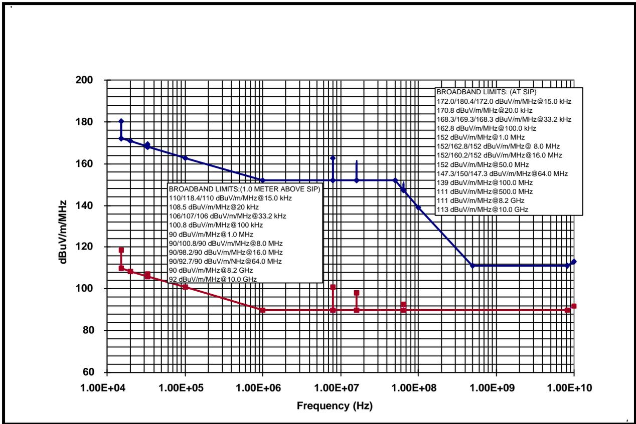
Figure 14 - Maximum LV Radiated Broadband Emissions
