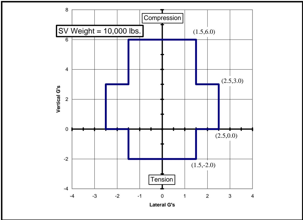
**Figure 21 - HLV Quasi-Static Load Factors**
