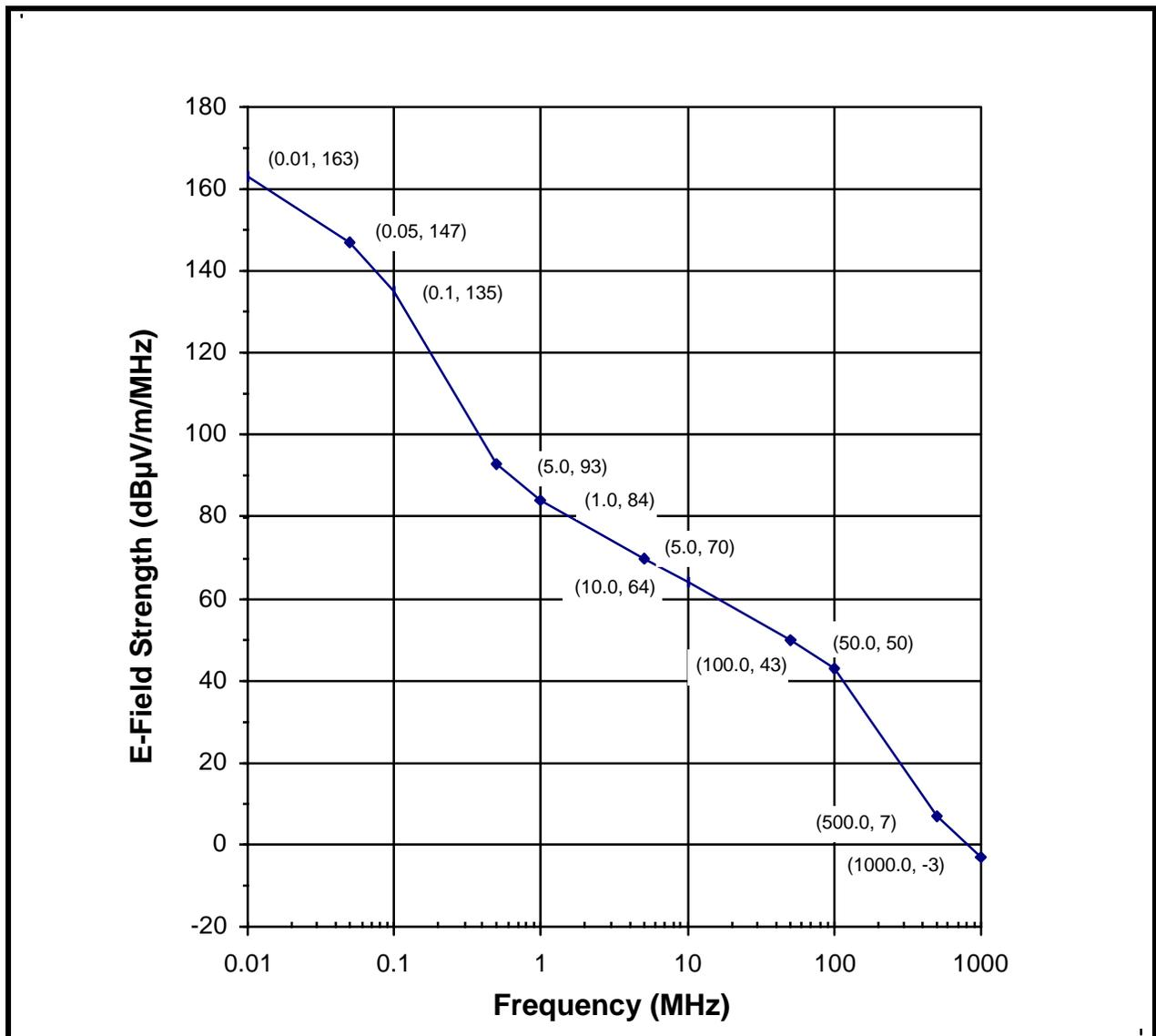
Figure 16 - E-Field Strength Derived Radially 1 cm from PLF Inner Surface
