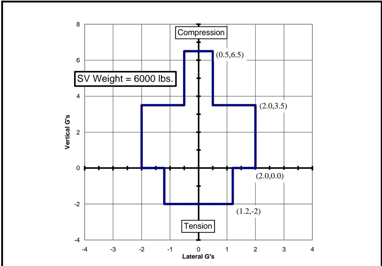
Figure 20 - MLV Quasi-Static Load Factors
