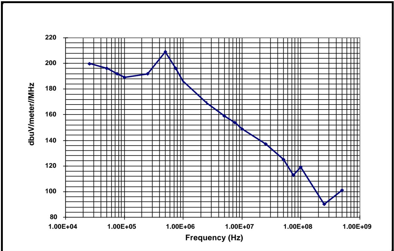
Figure 15 - Maximum Allowable Broadband Radiated E-Fields (ESD Source)
