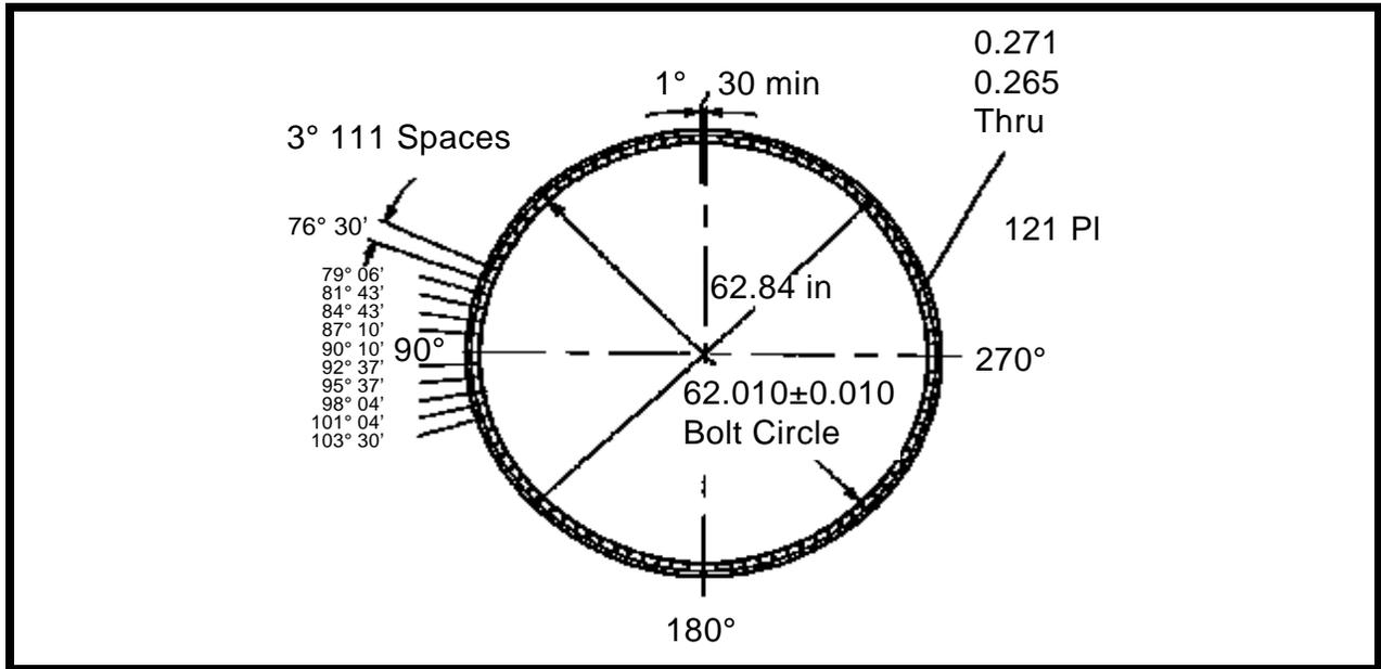
**Figure 3 - Small diameter (62.010'') payload interface**
