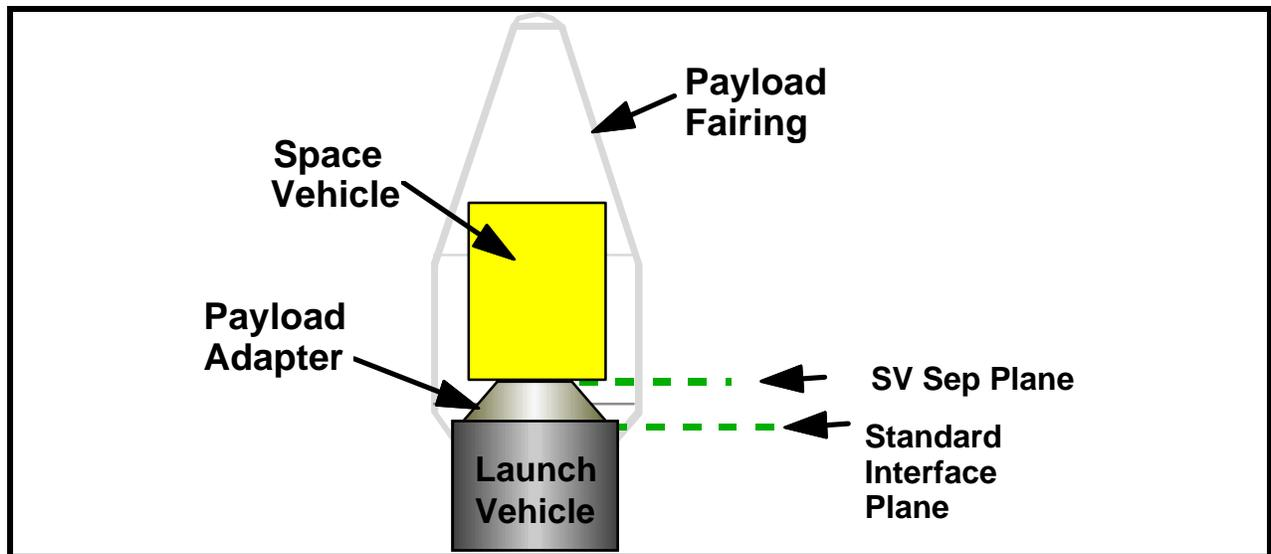
**Figure 2 - Standard Interface Plane - Relationship to SV**
