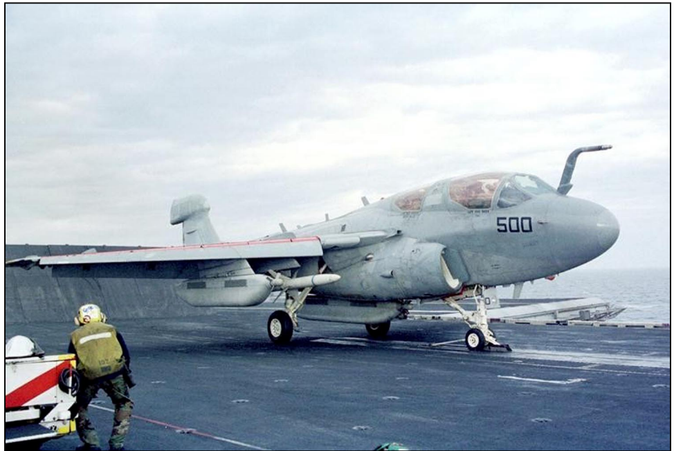
Figure 1: EA-6B with Jammer Pod and HARM Preparing for Launch from an Aircraft Carrier
