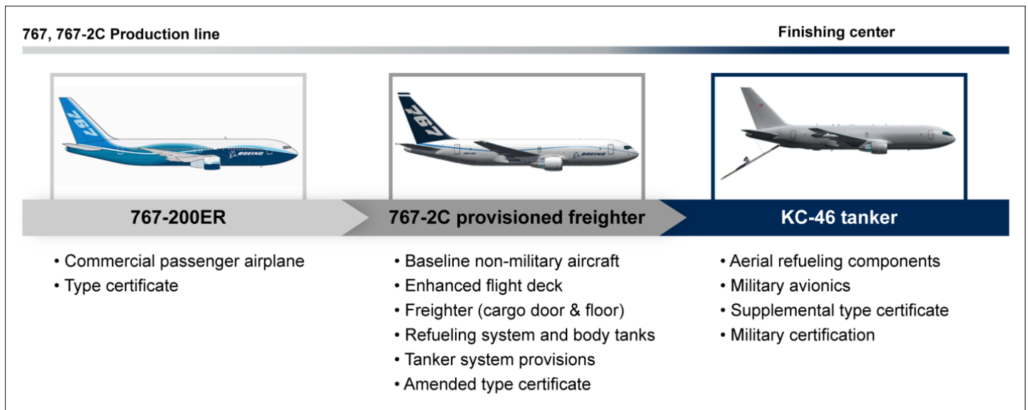
Figure 2: Conversion of a Boeing 767 into a KC-46 Aerial Refueling Tanker
