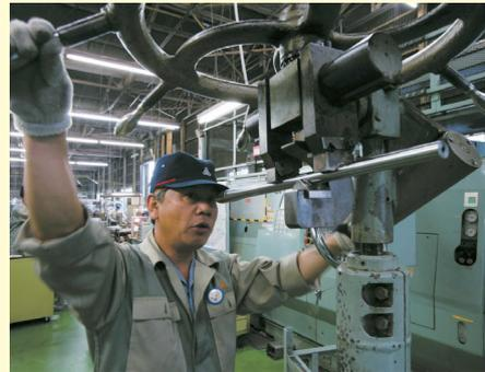
Worker engaged in eliminating distortion
