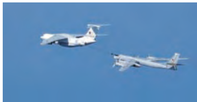
A Tu-95 long-range bomber undergoing mid-air refueling from an IL-78 aerial refueling tanker (September 8, 2011)
