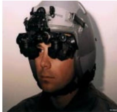
Figure 1. PNVG conceptual demonstrator (Patent Pending)
