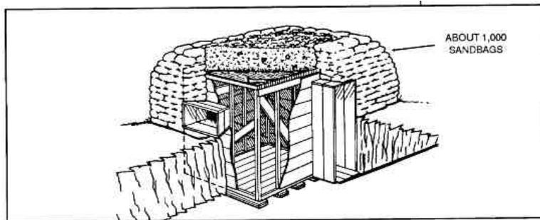
Figure 7-11. Cutaway view of a standard bunker.
