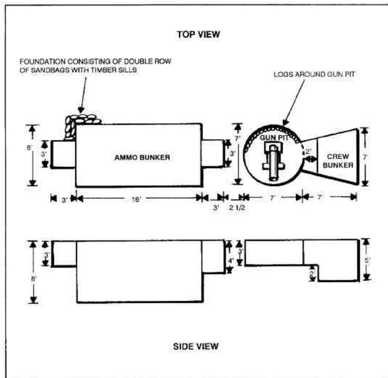
Figure 7-16. Dimensional drawing of heavy-mortar high-survivability position.
