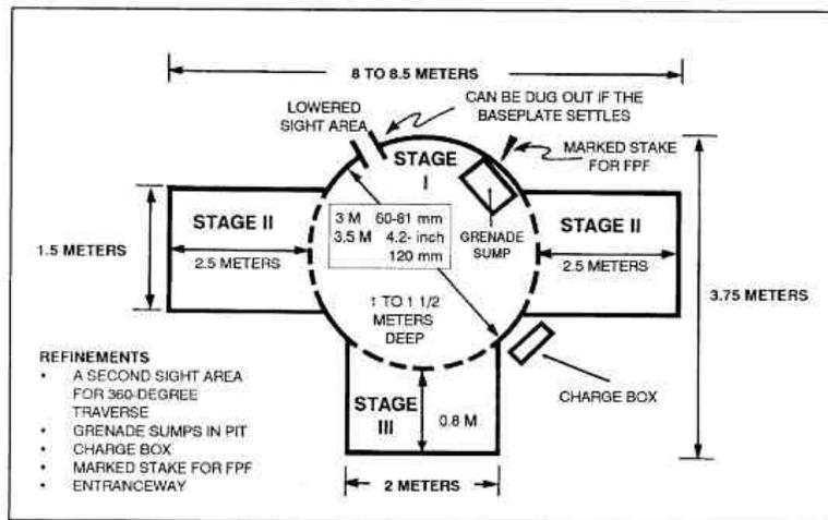
Figure 7-7. Mortar position (three stages of construction).
