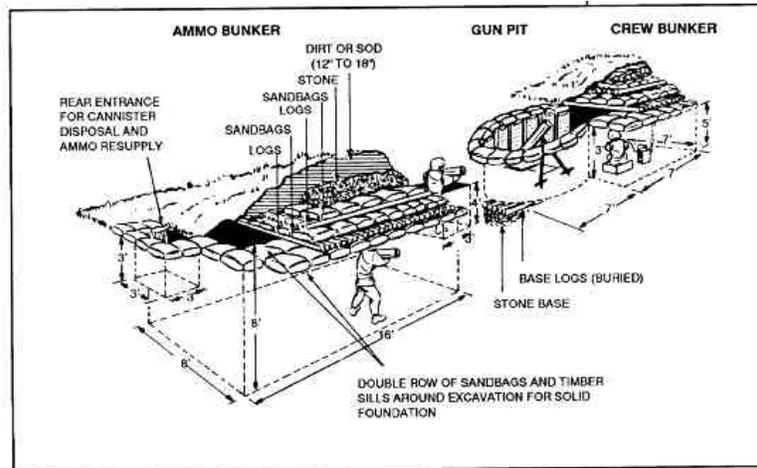
Figure 7-15. Cutaway view of heavy mortar, high-survivability position.
