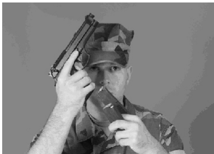
Figure 3-13. Condition 1 Reload - Removing a Partially Filled Magazine.
