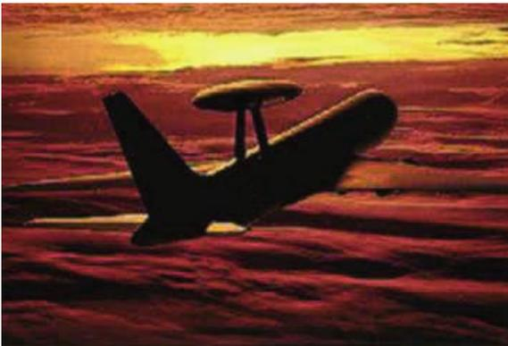
**The Airborne Warning and Control System electronically identifies friends through the use of identification friend or foe and selective identification feature interrogators.**
