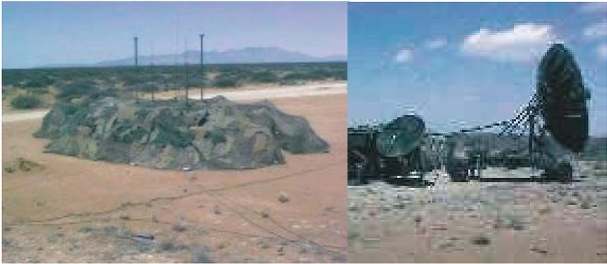
**The communications for the Theater Air Control System include line of sight (left) and satellite (right) systems.**
