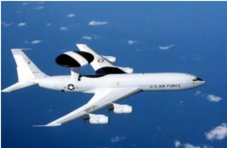
**E-3 Airborne Warning and Control System (AWACS) aircraft are a key element of C<sup>2</sup>.**
