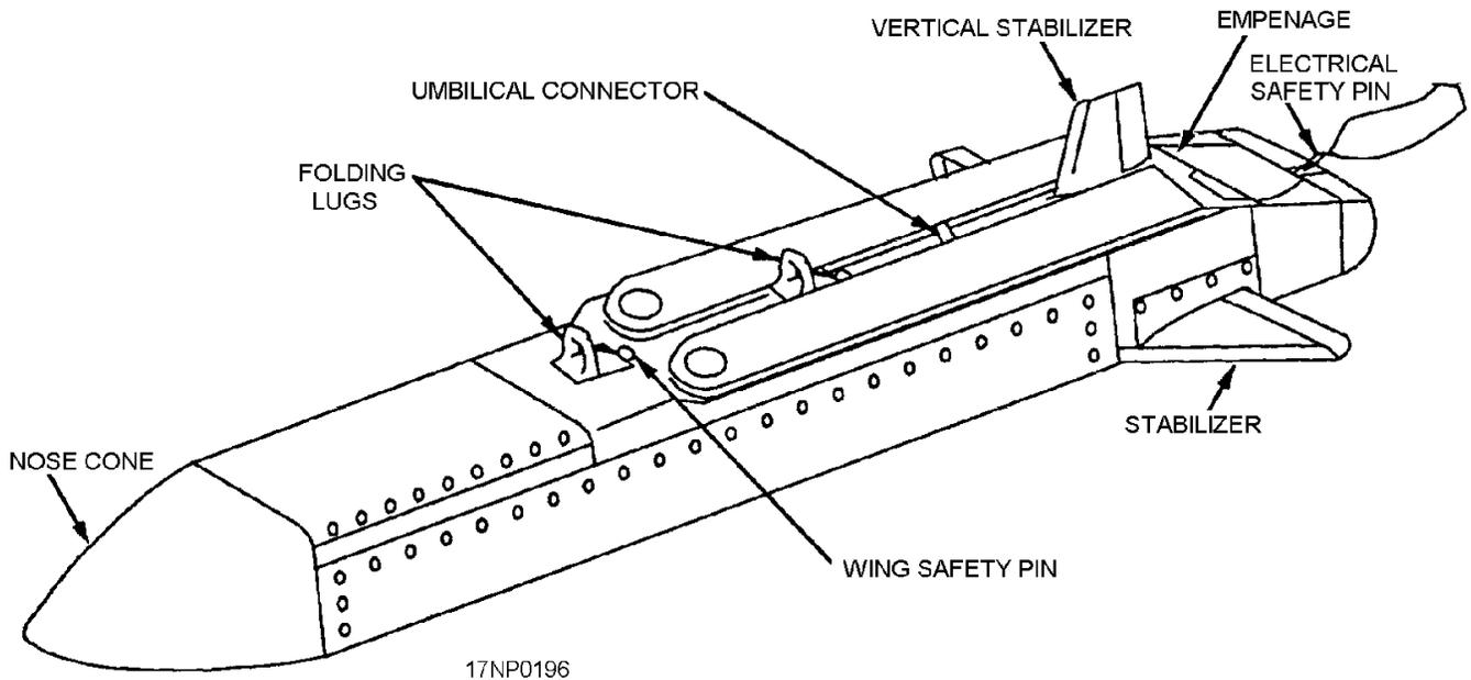
Figure 8-12.—Typical tactical air-launched decoy (TALD) component locations.
