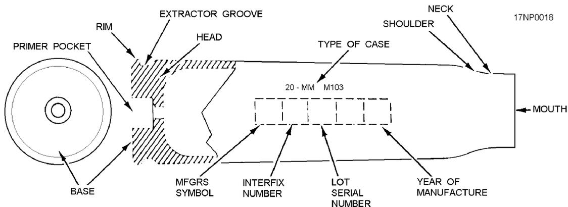
Figure 7-2.—M103 (brass) and M103B1 (steel) cartridge cases.
