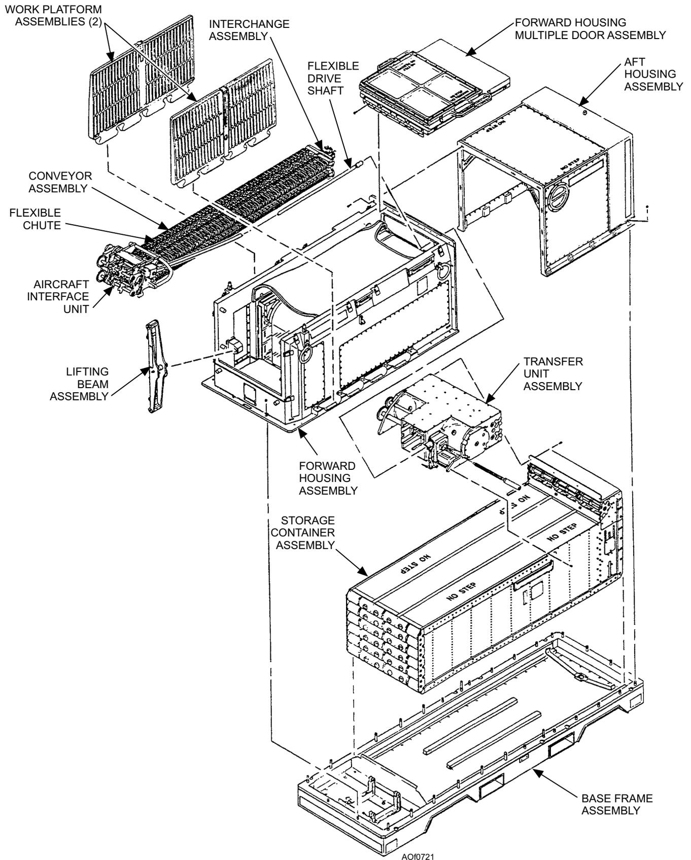
Figure 7-21.—Ammunition Loader.
