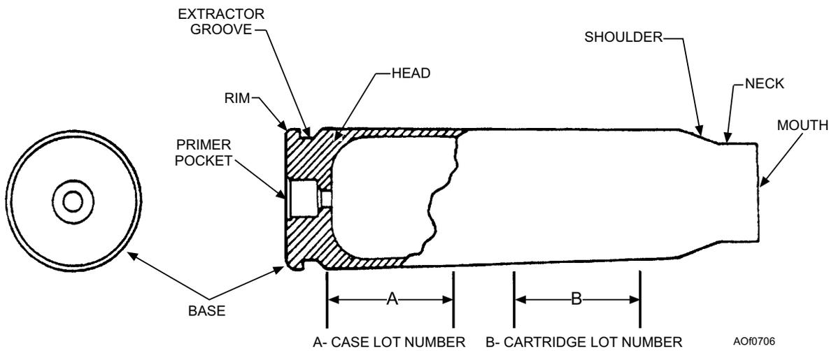
Figure 7-6.—M103 brass cartridge case and markings.
