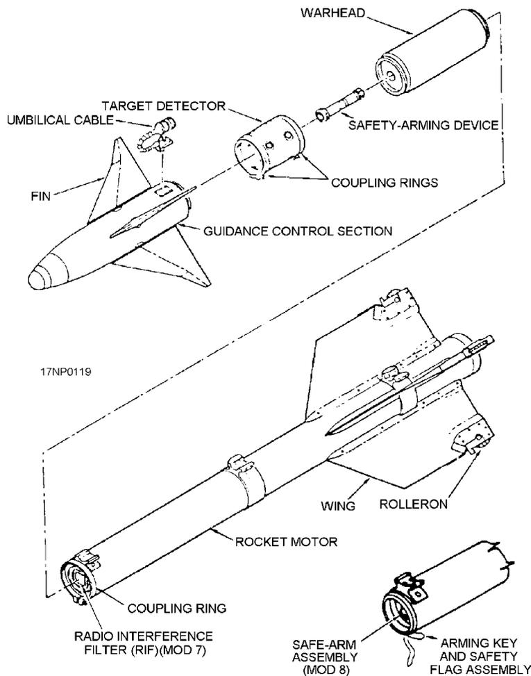
Figure 3-9.—AIM-9 series Sidewinder guided missile (exploded view).
