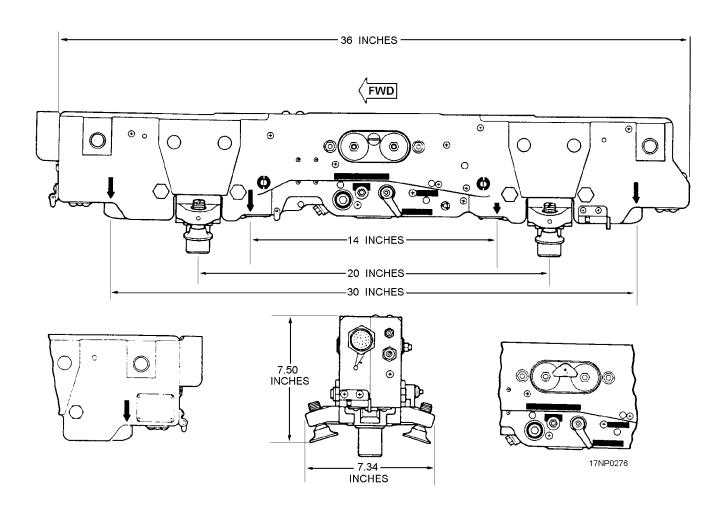
Figure 10-6.—BRU-32/A bomb ejector rack.
