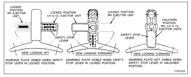
Figure 10-12.—Ejector unit safety stop lever.
