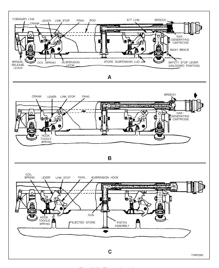
Figure 10-13.—Ejector unit operation.
