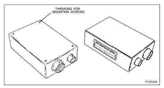
Figure 10-21.—Sequencer switch.
