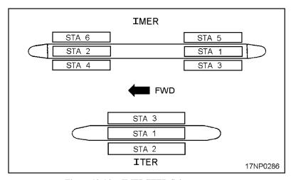
Figure 10-14.—IMER/ITER firing sequence.
