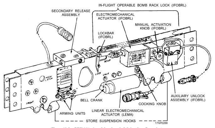
Figure 10-3.—BRU-14A aircraft bomb rack (left-hand configuration).
