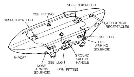
Figure 10-7.—BRU-33/A bomb ejector rack.
