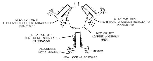
Figure 10-10.—IMER/ITER ejector unit locations.
