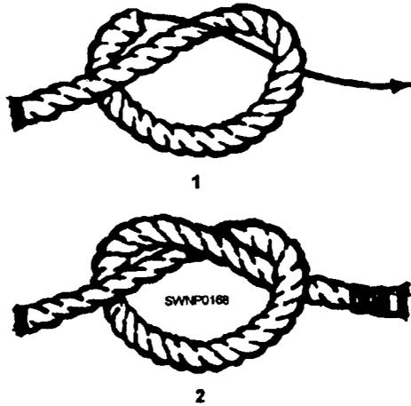
Figure 4-9.—Overhand knot.
