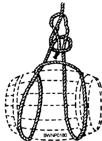
Figure 4-21.—Barrel hitch.
