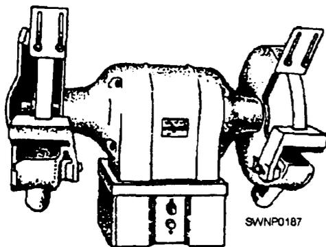
Figure 12-1.—The bench grinder, Eye shields have not been mounted.
