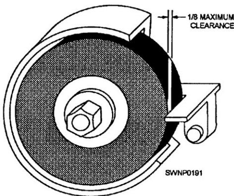
**Figure 12-5.—Properly spaced tool rest.**
