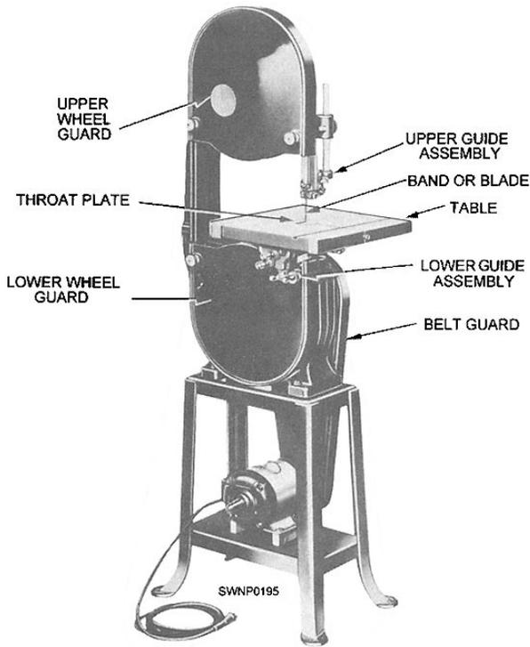
**Figure 12-9.—14-inch band saw.**
