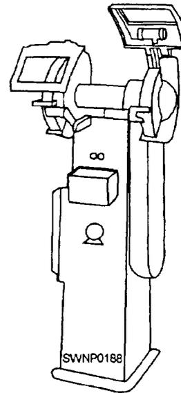
Figure 12-2.—The pedestal grinder (dry type).
