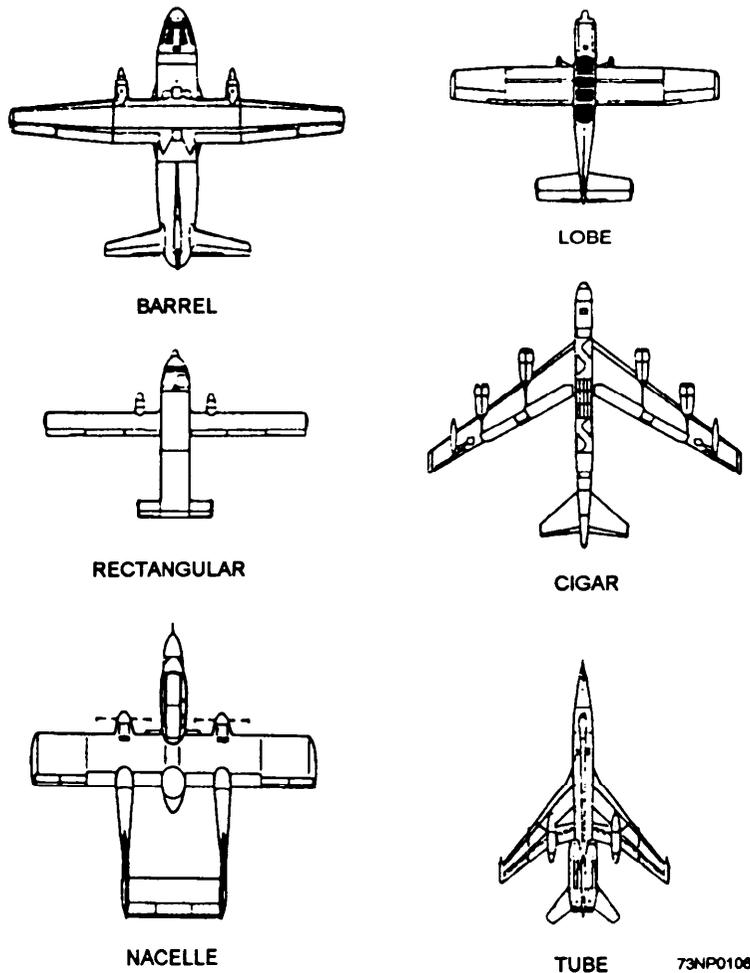
Figure 13-8.—Fuselage shapes
