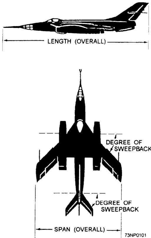
Figure 13-3.—Aircraft measurements.
