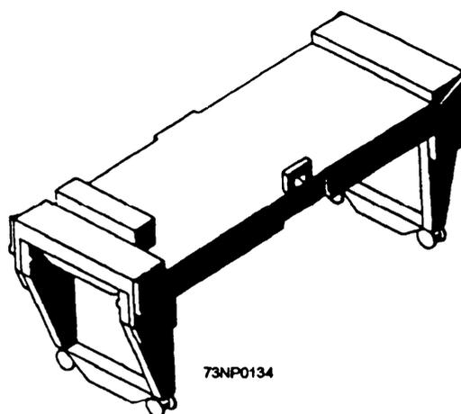
Figure 13-34.—Muckloader gantry.
