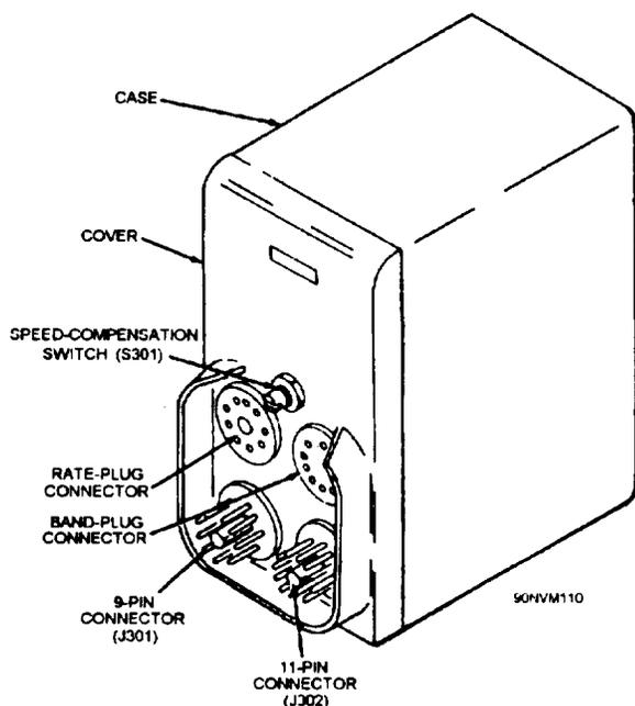
Figure 2-4.—Mk 21 Mod 0 firing mechanism.
