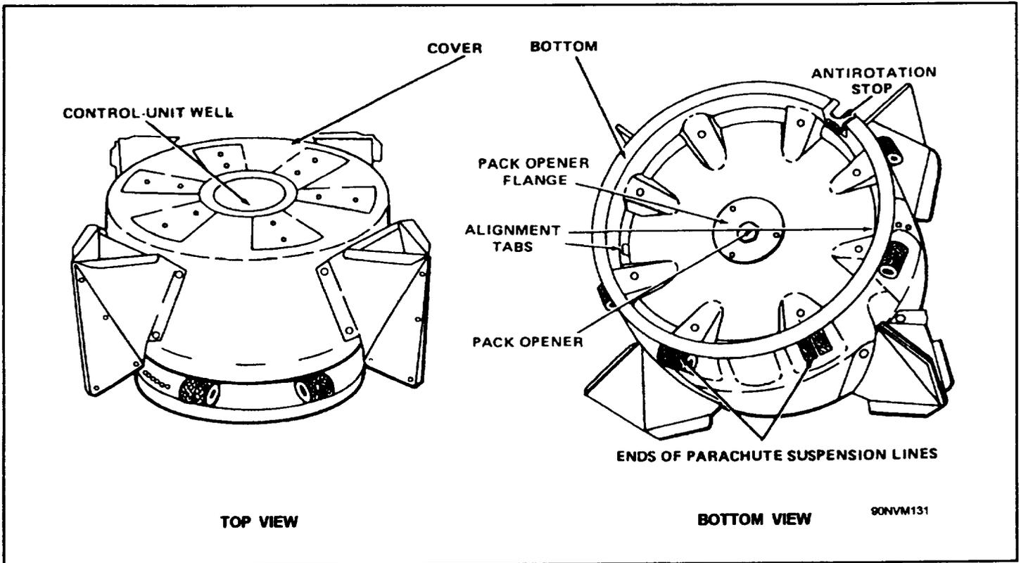
Figure 2-25.—Mk 36 Mod 0 parachute pack assembly.
