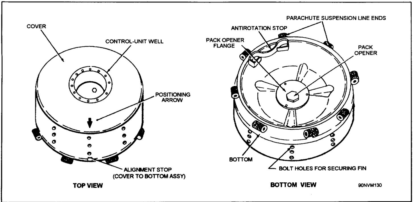
Figure 2-24.—Mk 35 Mod 0 parachute pack assembly.
