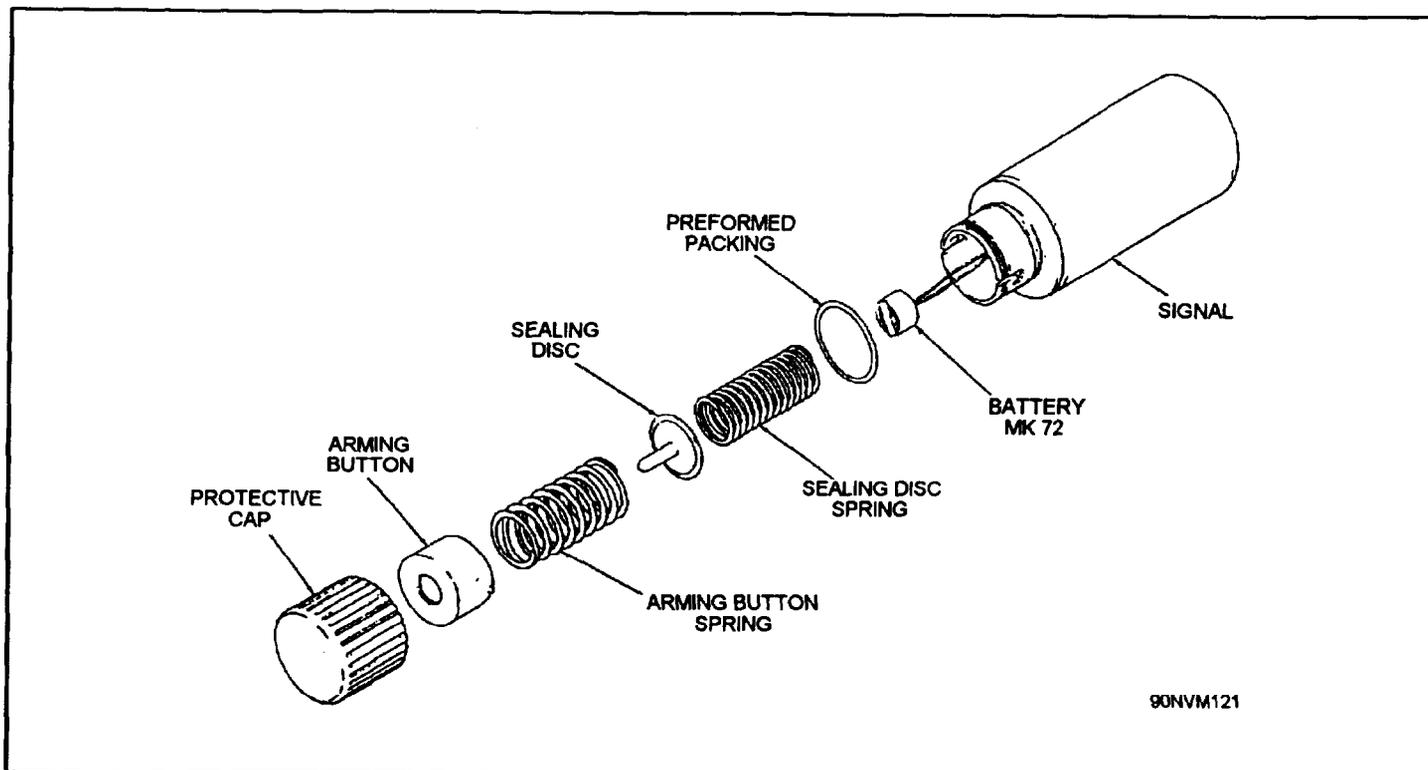
Figure 2-15.—Mk 125 Mod 0 smoke and illumination signal.
