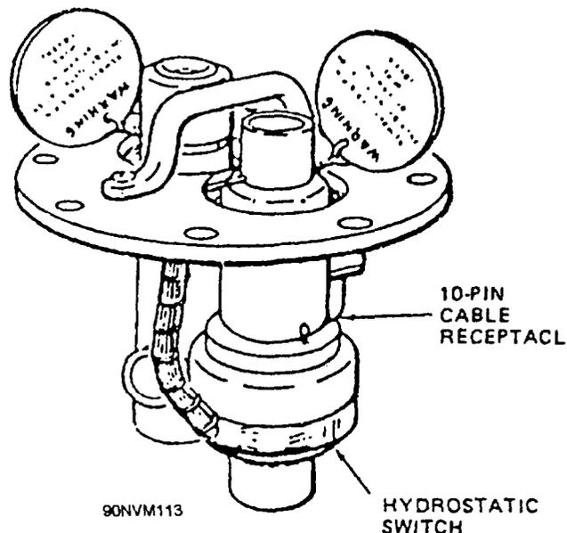
Figure 2-7.—Mk 5 Mod 1 ET arming device.
