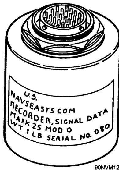
Figure 2-19.—Mk 25 Mod 0 signal data recorder.
