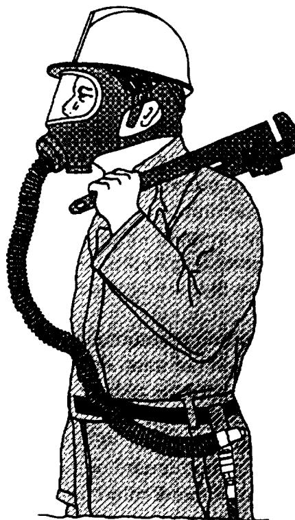
Figure 1-31.—Supplied-air respirator hose-line mask.
