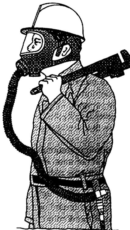
Figure 1-31.—Supplied-air respirator hose-line mask.
