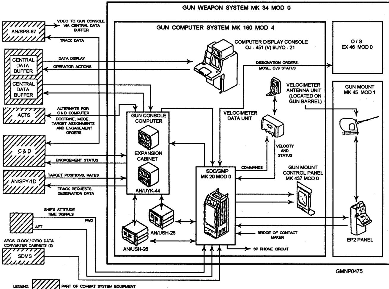
Figure 10-11.—Functional interface of the Mk 34 GWS.
