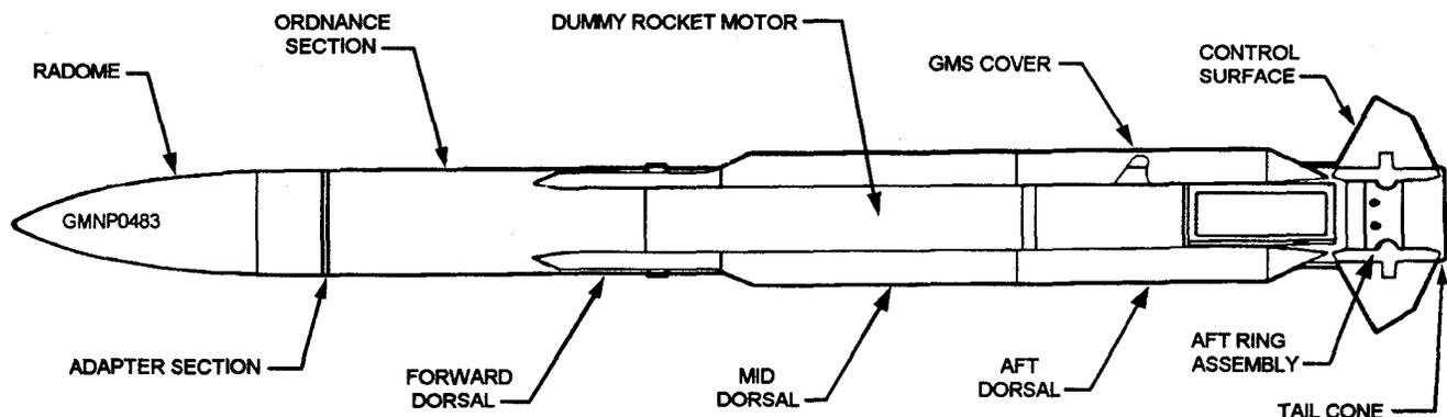
Figure 10-19.—Mk 60 Mod 6, 7 GMTR for Standard missile systems.
