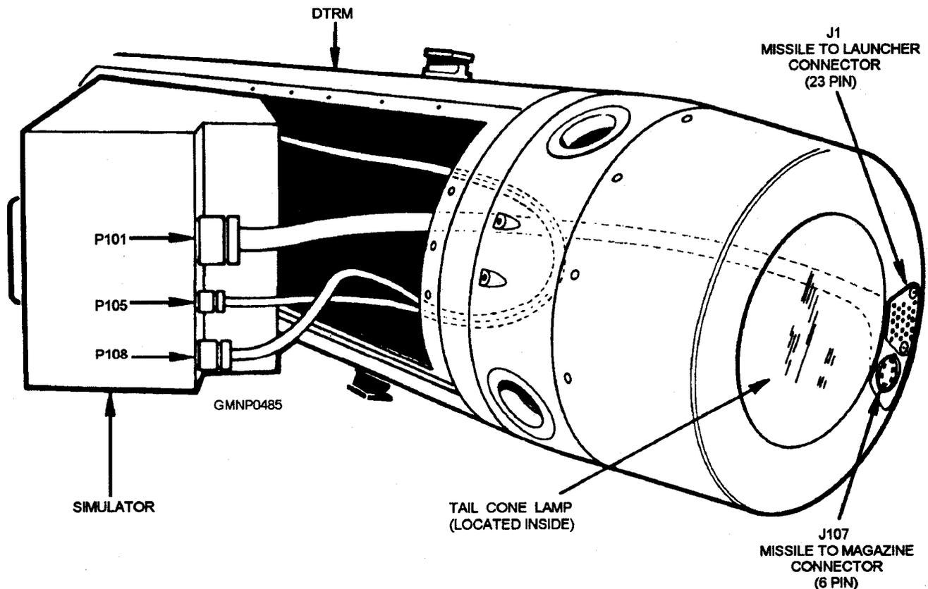
Figure 10-21.—Tail cone assembly components and simulator removal.
