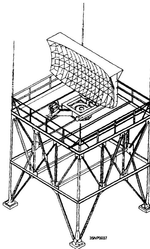
Figure 2-45.—AN/GPN-27(ASR-8) air surveillance radar.
