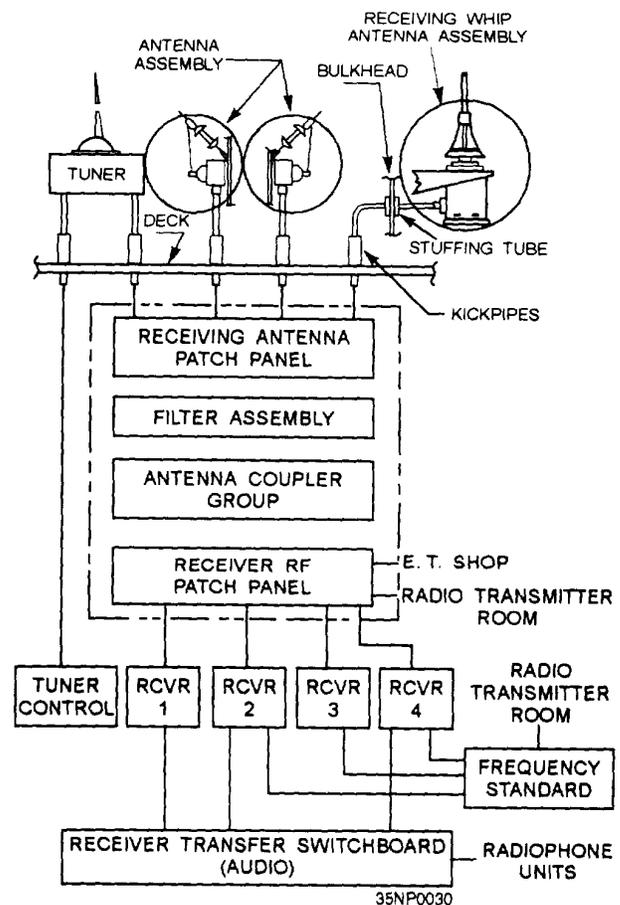
Figure 2-38.—Receive signal distribution system.
