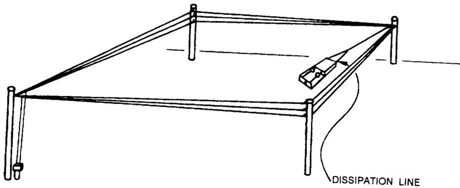
**B. NON - RESONANT HORIZONTAL THREE - WIRE RHOMBIC**
