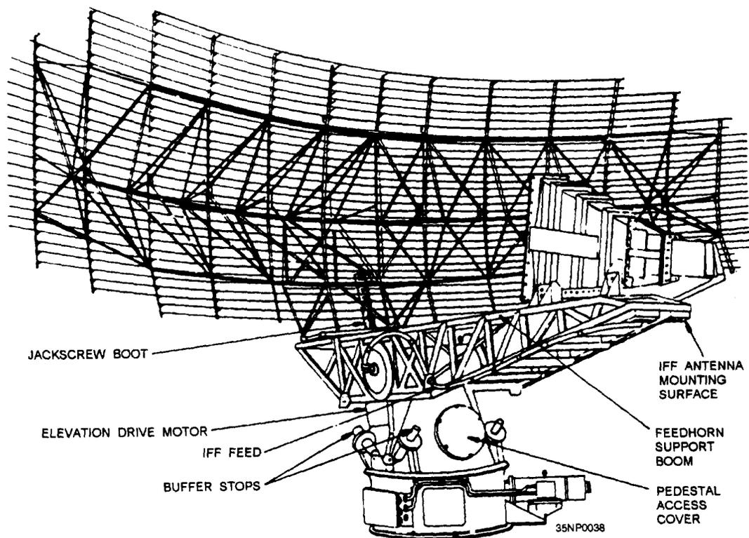
Figure 2-46.—AS-3263/SPS-49(V) antenna.
