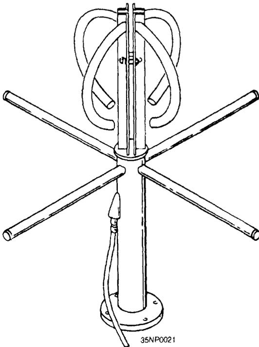
Figure 2-29.—AS-2815/SSR-1 fleet broadcast satellite receiving antenna.
