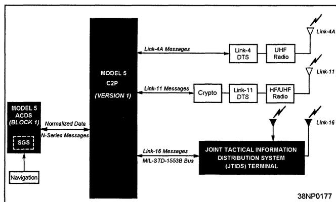
Figure 7-6.—The Link-16 Model-5 ACDS system block diagram.
