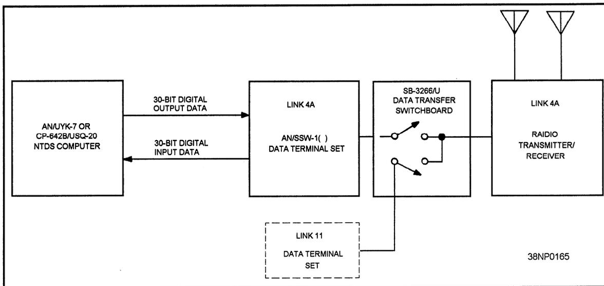
Figure 6-1.—The shipboard Link-4A CDS system.
