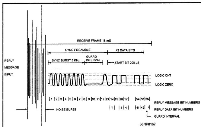
Figure 6-3.—The Link-4A reply message format.
