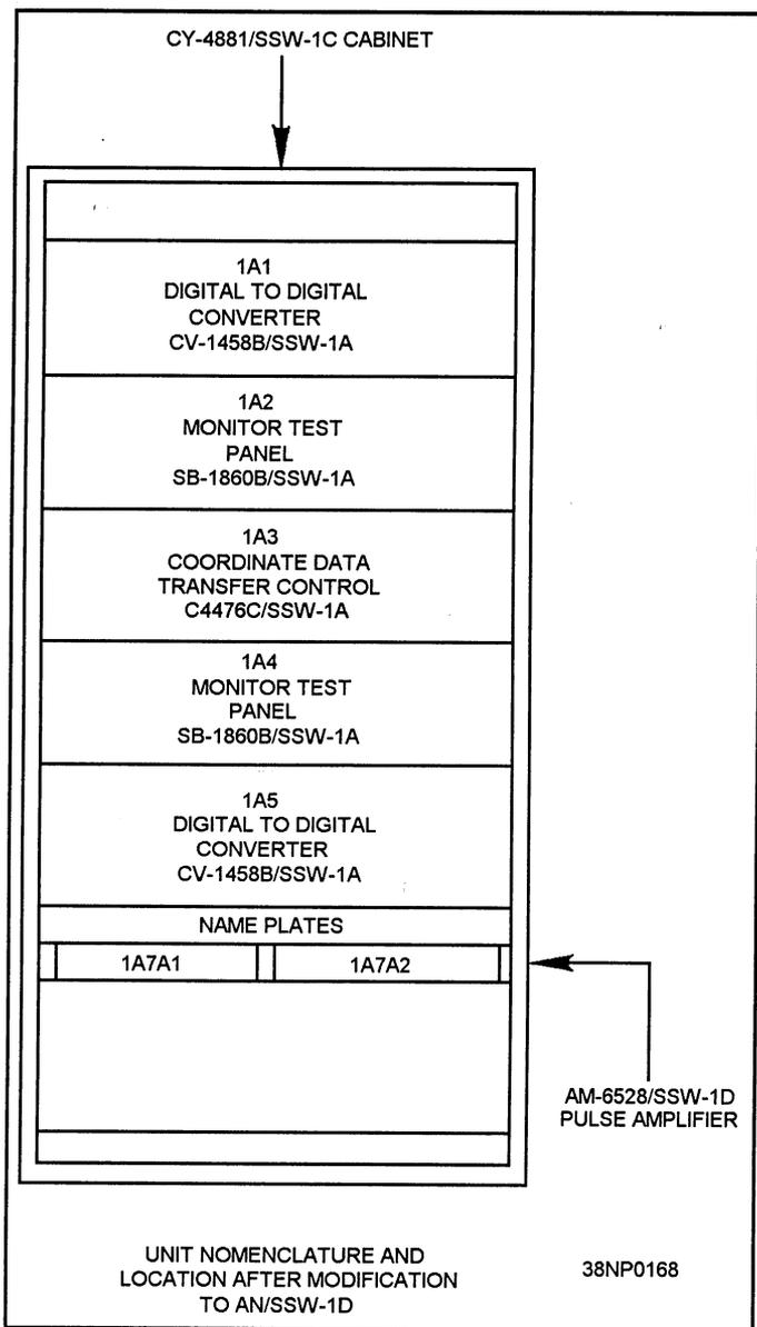
Figure 6-4.—The AN/SSW-1D/E data terminal set.
