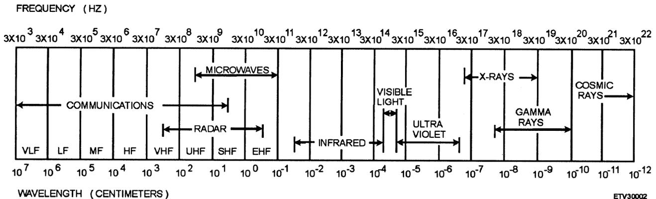
Figure 1-2.—Frequency spectrum.
