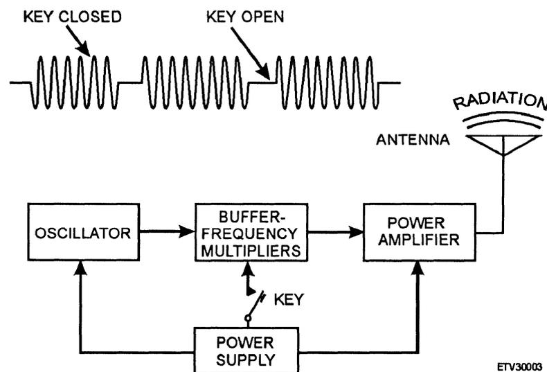
Figure 1-3.—Continuous-wave transmitter.
