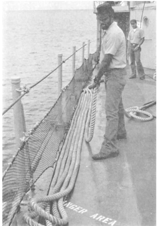
Figure 3-4.—Faking down a line. 80.22
