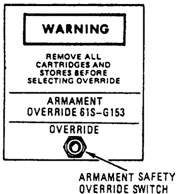
Figure 7-10.-Armament safety override switch.
