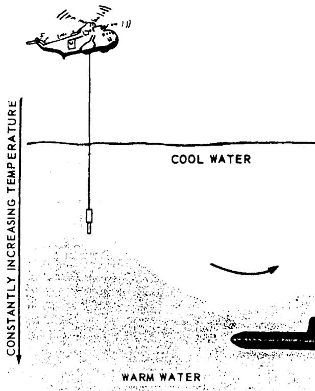
Figure 4-3. The effect of a positive thermal gradient.
