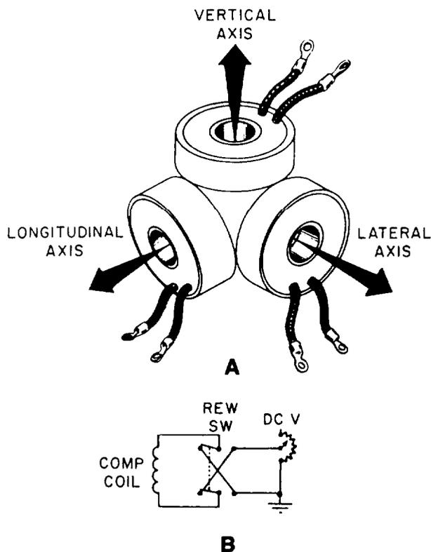
Figure 4-25.-A. Arrangement of compensating coils.
