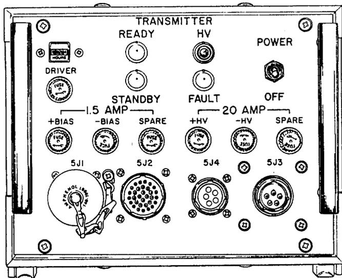
Figure 4-19. Sonar transmitter.
