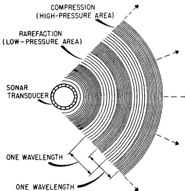
Figure 4-1. Sound waves produced in water by a transducer.
