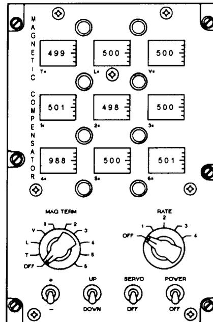
Figure 4-28.—Compensator control-indicator.
