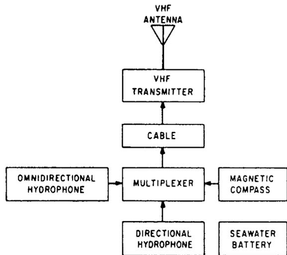
Figure 4-31.-Block diagram of the DIFAR sonobuoy.
