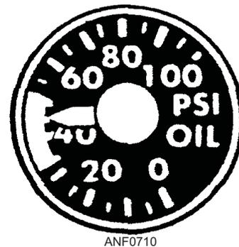
Figure 7-10.—Oil pressure indicator.
