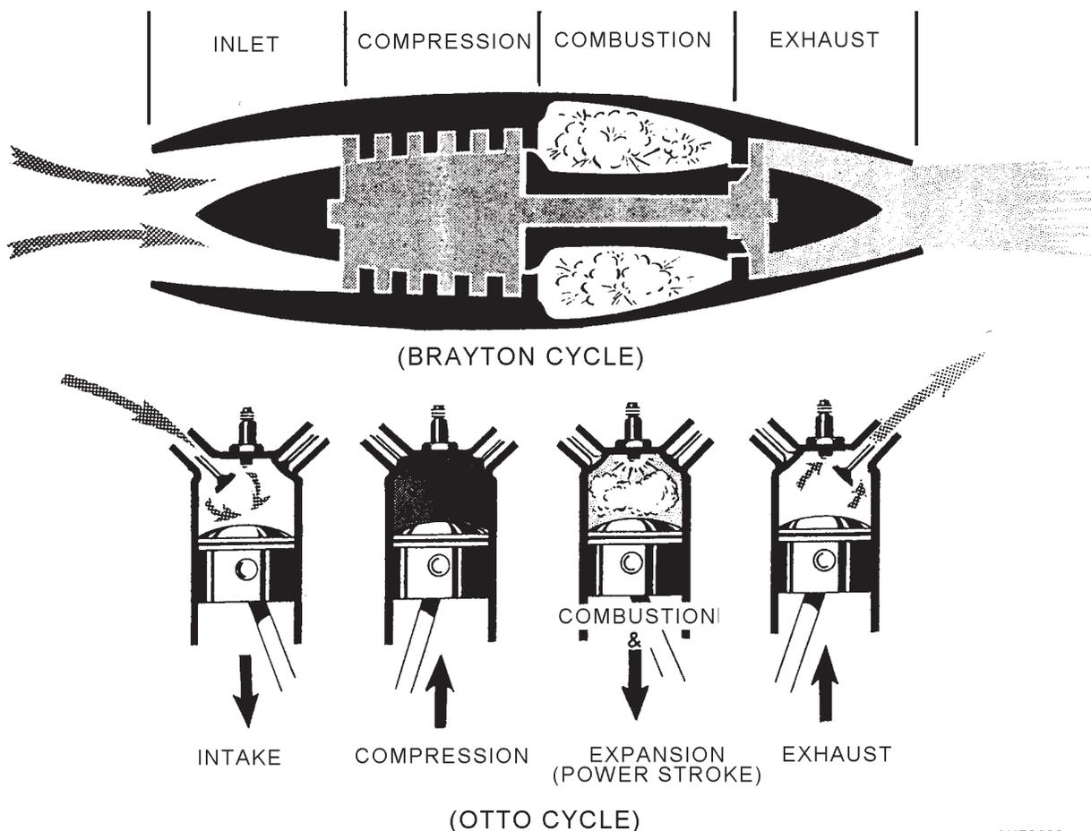
Figure 6-20.—A comparison of turbojet and reciprocating engine cycles.
