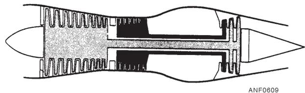
Figure 6-9.—Dual rotor turbine for split spool compressor.
