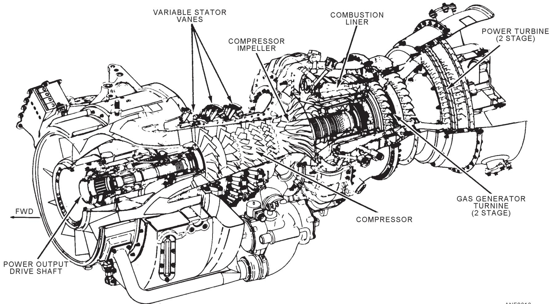
Figure 6-16.—Turboshaft gas turbine engine.
