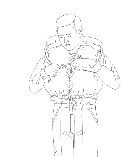
A. LIFE PRESERVER DONNED JACKET TIED AT UPPER CHEST AND WAIST: TIE PULLED SNUG, SNAP HOOK BEING FASTENED INTO RING ON CHEST STRAP.
