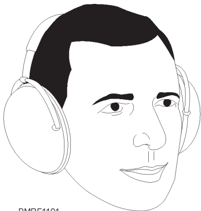
Figure 11-1.—Circumaural (Mickey Mouse) type of ear protector.
