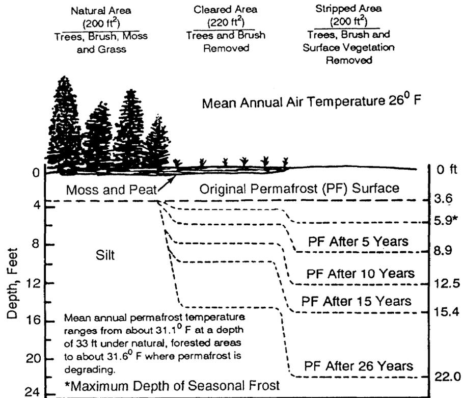
Figure 12-8. Permafrost degradation under different surface treatments.
