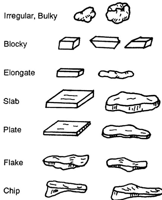
Figure 1-13. Crushed shape.
