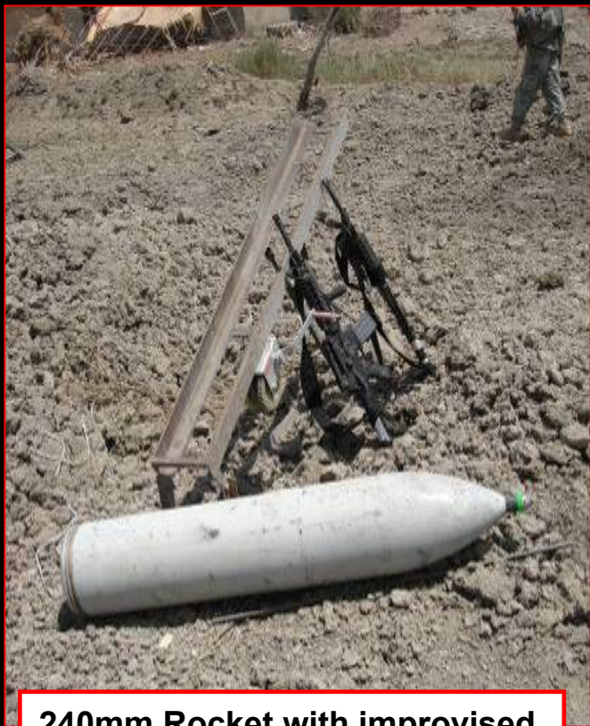
240mm Rocket with improvised launch device
