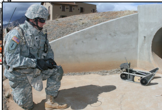
Searching culvert with Small Unmanned Ground Vehicle
