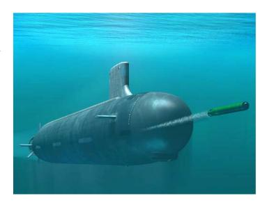
Mk 48 Mod 7 CBASS upgrades the Mk 48 ACOT-GCB with a new sonar and improves torpedo effectiveness through future software upgrades, called Advanced Processor Builds (APB). CBASS is a co-development program with the Australian Navy.
