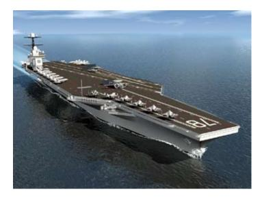
CVN 21 is designed to increase the sortie generation capability of embarked aircraft and have increased self-defense capabilities when compared to current aircraft carriers.
