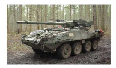
The MGS provides the crew with levels of protection against small-arms, fragmenting artillery, mines, and rocket-propelled grenades. Rocket-propelled grenade protection is provided by add-on Slat armor (flat steel stock arranged in a spaced array) not shown in photo.
