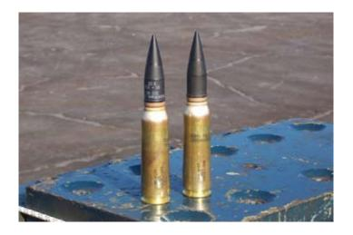
• The PELE cartridge is intended to be compatible with F-15, F-16, and F-22 aircraft.
