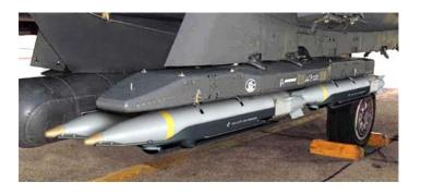
GPS satellite positioning error data and broadcasts target location corrections to the SDB through the F-15E data link prior to weapon release.
