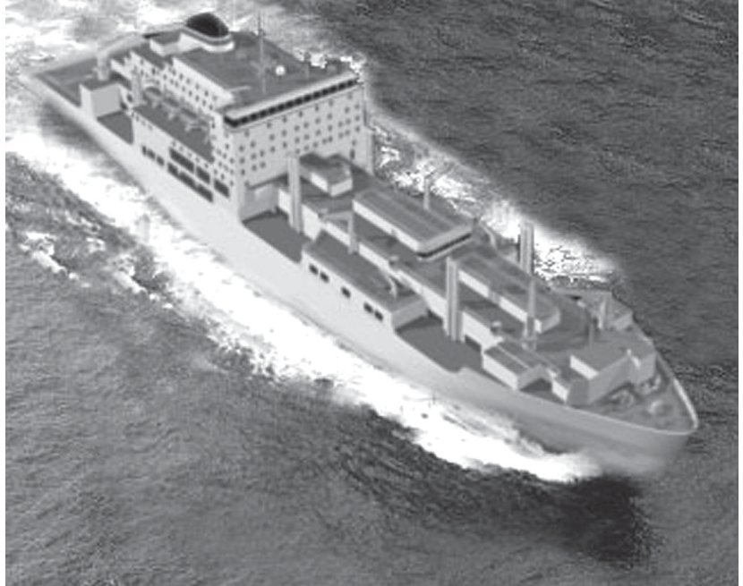
The T-AKE will primarily function as a shuttle ship, ferrying cargo and ammunition between port and a larger, consolidating replenishment ship.
