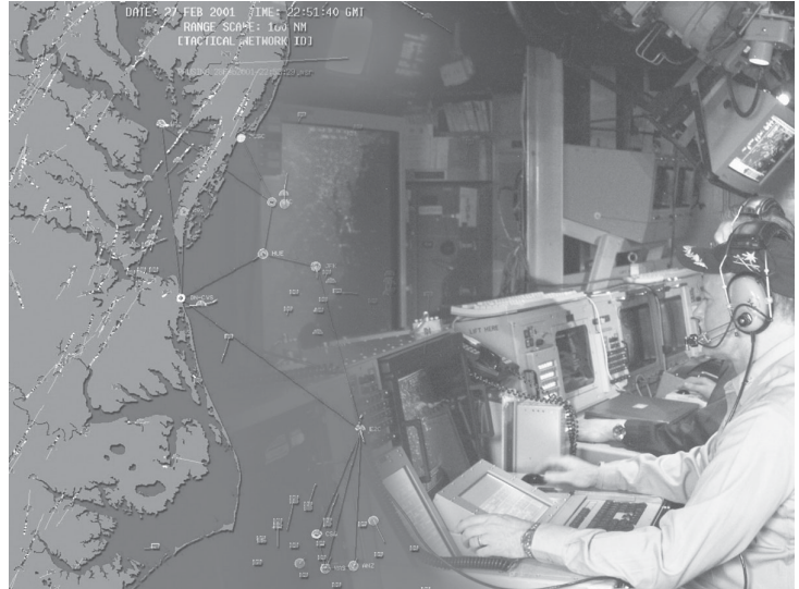
The CEC is a system of hardware and software that allows ships and E-2C aircraft to share radar data on air targets.
