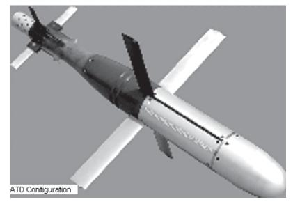
The Army will use PGMM to incapacitate personnel in standard brick over block masonry structures, collapse earth and timber bunkers, and defeat stationary lightly armored vehicles or incapacitate personnel inside.
