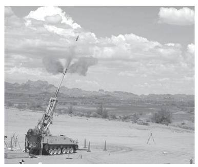
Between September 2003 and January 2004, the Army conducted live fire tests of the NLOS-C demonstrator at Yuma Proving Grounds, Arizona, to examine whether a lightweight chassis is stable enough to support a 155mm cannon during firing.
