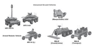
The UGVs within the Future Combat System program consist of three categories or classes: Class I – light vehicles, Class II – medium vehicles, and Class III – heavy vehicles.
