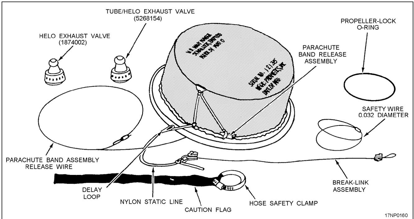
Figure 5-6.—Mk 31 Mod 0 torpedo air stabilizer.
