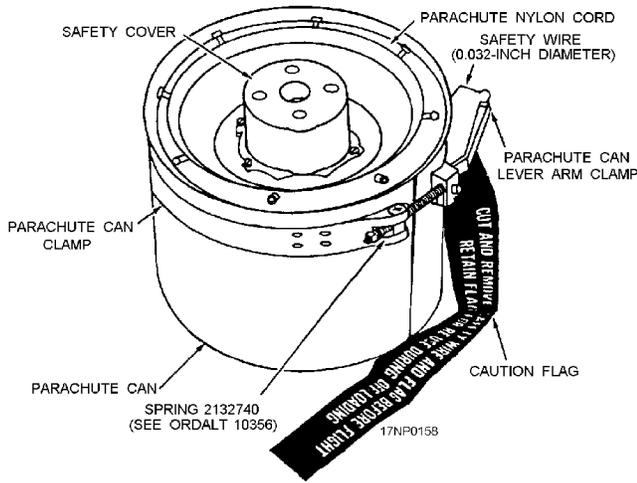
Figure 5-4.—Mk 28 Mod 2 torpedo air stabilizer.
