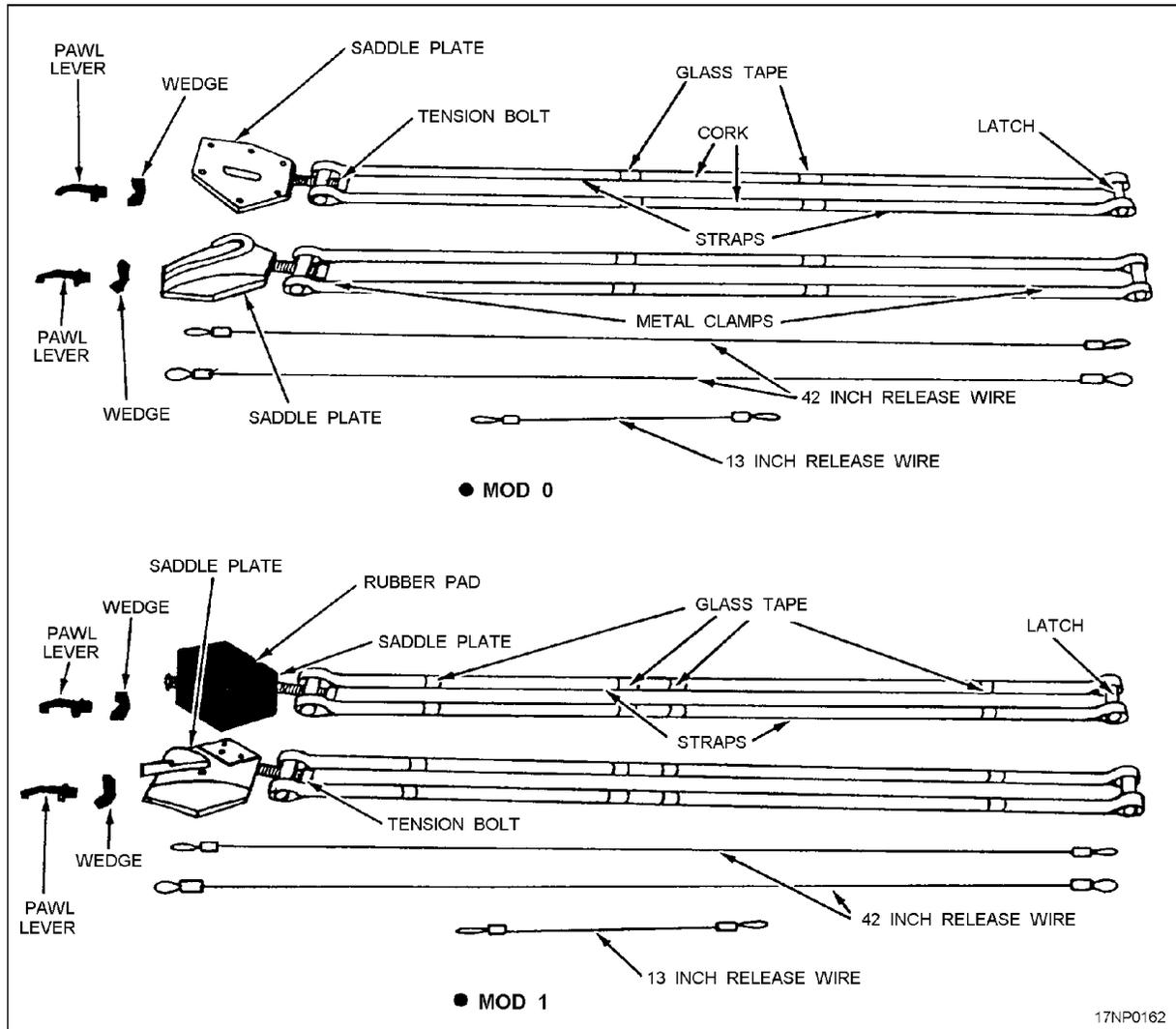
Figure 5-8.—Mk 78 Mod 0 and Mod 1 suspension band assemblies.
