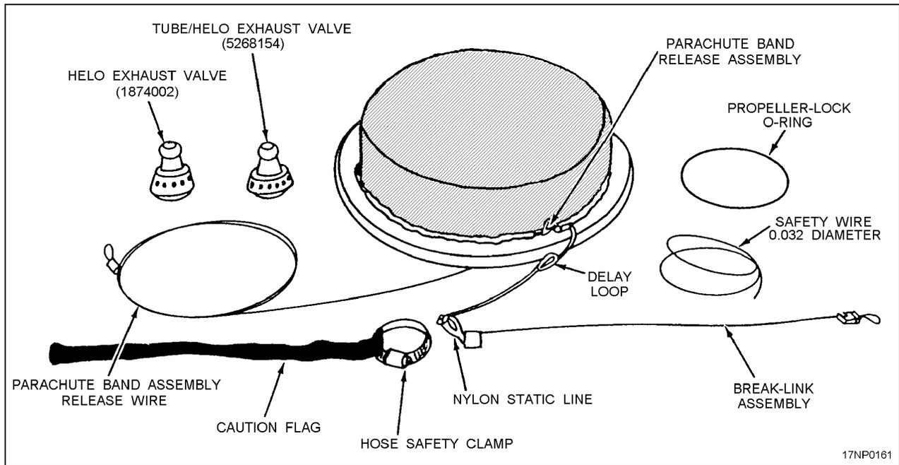
Figure 5-7.—Mk 31 Mod 1 torpedo air stabilizer.
