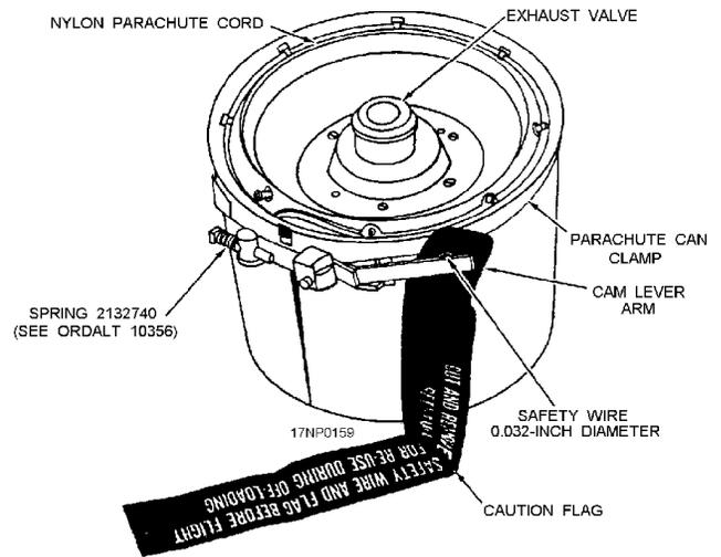
Figure 5-5.—Mk 28 Mod 3 torpedo air stabilizer.
